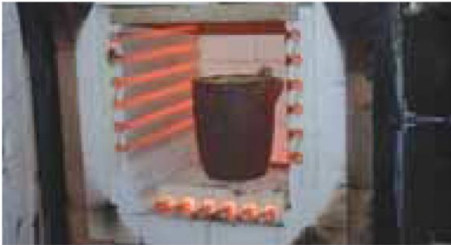
Furnace walls and electric wils.
