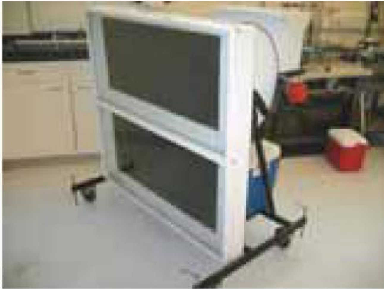
Solar heat collector.
