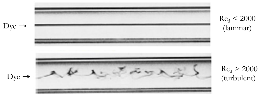
Figure 18. Images of a tracer dye in laminar and turbulent pipe flow. Flow from left to right. (From http://olivier.granier.free.fr )
