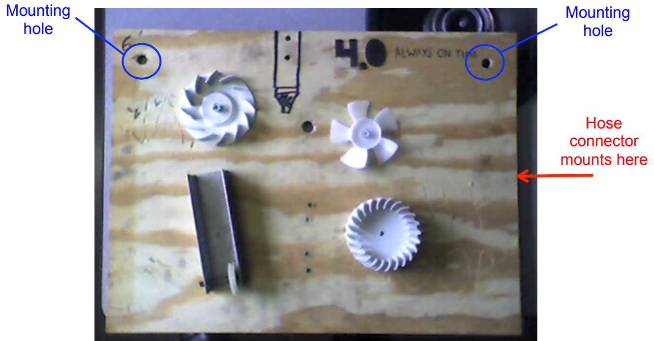
Figure 29. Picture of mounting board, with some turbine wheels shown for scale.
